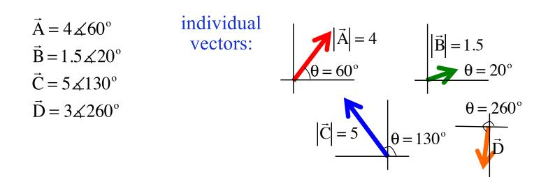
• *Given* information about the magnitude (length) and orientation (angle) of each vector, use a **ruler** and a **protractor** to draw vectors to scale.
